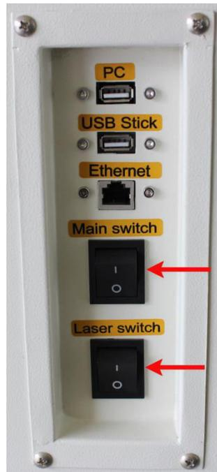
If all covers are closed, immediately after being switched on, the device starts the referencing process. When the referencing process is completed correctly, an acoustic signal sounds and the device is ready for operation. The operation panel will display the home screen when the laser is completed resets.
