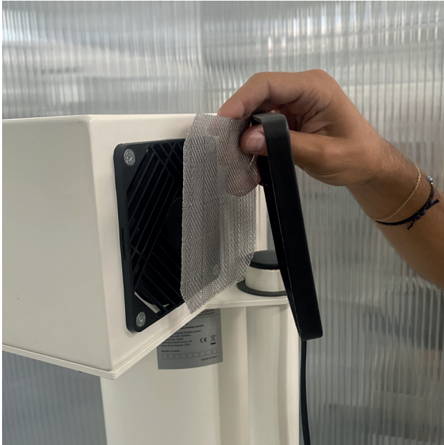
Fig. 7.3.3 - Fan filter dust check and cleaning
