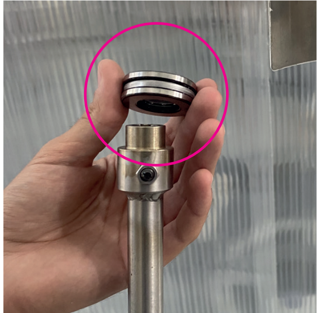
Fig. 7.3.4 - Mixer bearing lubing
